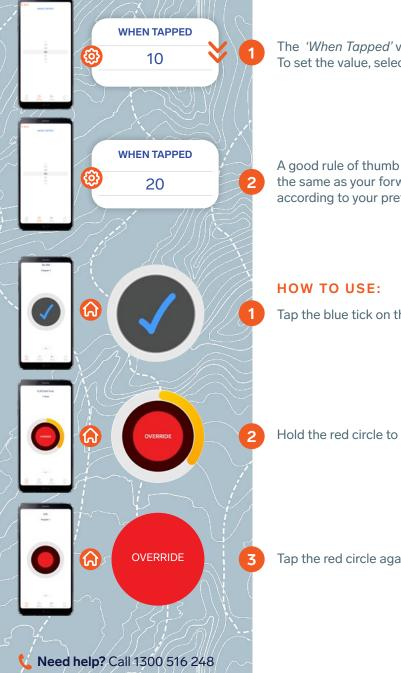
The *'When Tapped'* value controls the manual override brake response. To set the value, select *'When Tapped'* under Override in program screen.
